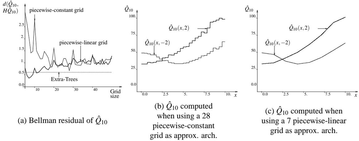
Figure 7: Fitted  $Q$  iteration with basis function methods. Two different types of approximation architectures are considered: piecewise-constant and piecewise-linear grids. 300 episodes are used to generate  $\mathcal{F}$ .
