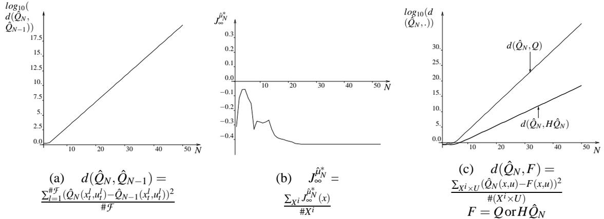
Figure 15: Fitted  $Q$  iteration algorithm with basis function methods. A  $12 \times 12$  piecewise-linear grid is the approximation architecture considered. The sequence of  $\hat{Q}_N$ -functions *diverges to infinity*.
